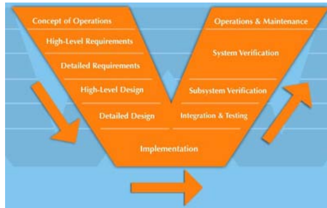
Figure 2: Typical Systems Engineering Process “V” Diagram
